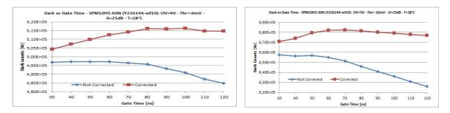
We select as optimal Gate Time  $\tau = 90$  ns. The SiPMs have been characterized by using the characterization facility available at the INAF [1] - [2] and taking care of having the best illumination conditions, that means avoiding the system saturation and maintaining a sufficient signal on the NIST calibrated photodiode.
